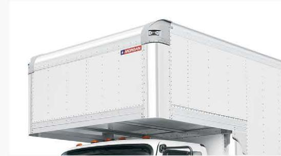
Innovative design of our "PEAK" overcab storage compartment maximizes cargo area, and provides out-of-the-way protection for delicate cargo. Optional skylights also enhance overall visibility.
