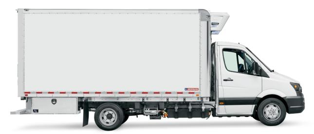
Chassis: Workhorse W4 CC Chassis GVWR: **14,330 lbs** Body Model: VCR08516096 Body Dimensions: **16'L x 85"H x 96"W**  Chassis Weight: **7,020 lbs** Body Weight w/Options: **3,000 lbs** Total Unit Weight: **10,020 lbs** Available Payload: **4,310 lbs**
