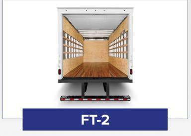
3/8" plywood sides and partially exposed wood slats to provide varying degrees of sidewall protection, 1/2" plywood front.
